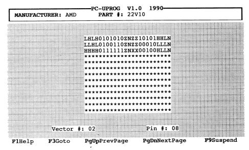
The vector buffer is arranged in rows (corresponding to vector number) and columns (corresponding to pin number). Each vector consists of the test condition codes for each pin of the device. The valid test condition codes are:
