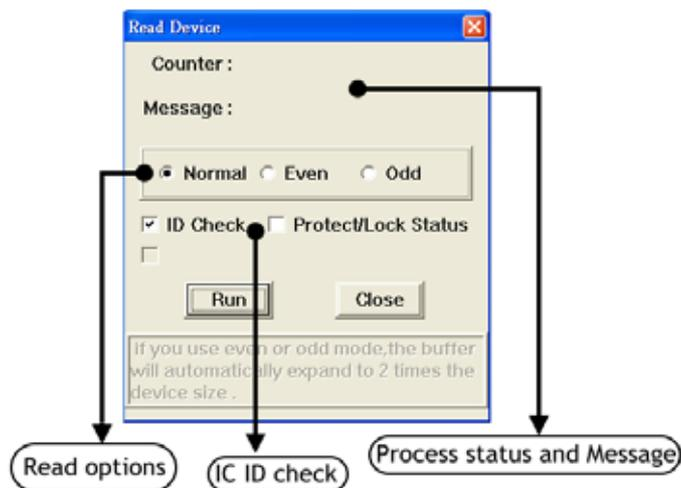
☆ After Read operation, suggest user to double-check to confirm checksum and the data read are all correct.
