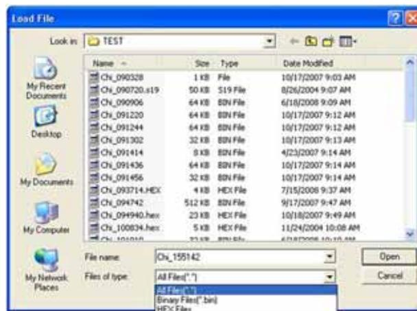
Function of file loading is similar to that under Windows environment. Enter the file name to be downloaded and click "Open", the named file will be loaded to programmer buffer. **Note: Disk drive and file path must be correct.** Select and click the correct drive and folder that the file located to. If it cannot be operated by mouse, apply <TAB>, <UP>, <DOWN>, and <ENTER> keys for selecting and confirming.
