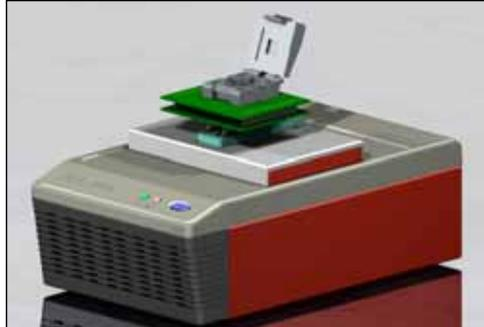
**Note:** While inserting ADAPTER or CONVERTER onto DIP ZIF socket, please have it close to bottom of the socket ( toward the YES key), and you should insert ADAPTER/CONVERTER by following direction as the picture shows.
