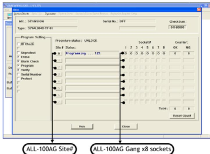
Up to 8 sets of ALL-100AG Gang Programmer can be connected to PC through USB interface, this is so call "Multiple ALL-100AG Gang Setup". Each ALL-100AG Gang can program 8 ICs. One PC with 8 sites of ALL-100AG Gang setup can program  $8 \times 8 = 64$  ICs.
