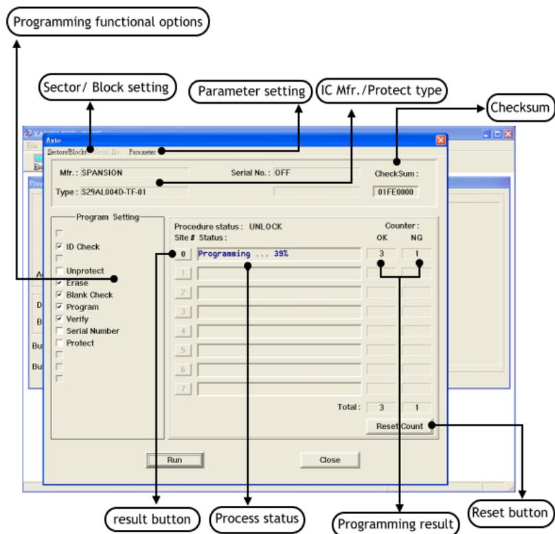
☆ Different IC product type might have different programming functional setting and parameter setting. User needs to refer IC data sheet for proper settings of programming functions and programming parameters.
