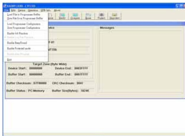
(1) Click “Load File to Programmer Buffer” in File to load data file:
