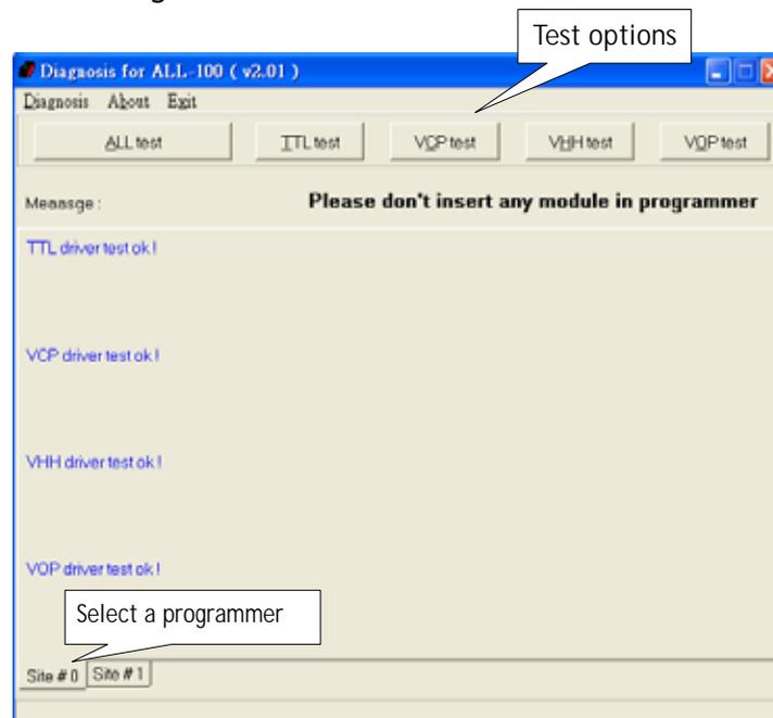
The diagnostic includes ALL Test, TTL Test, VCP Test, VHH Test, VOP Test; if it passes ALL-test, you will see result like the picture.
