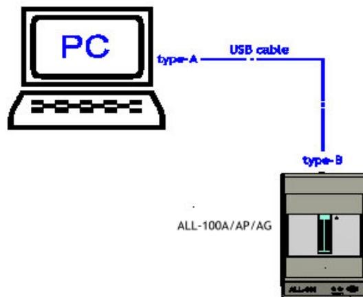
Connect the Type B end of USB cable to the USB Type B connector at rear panel of programmer, connect the Type A end of USB cable to the USB Type A connector on the PC.
