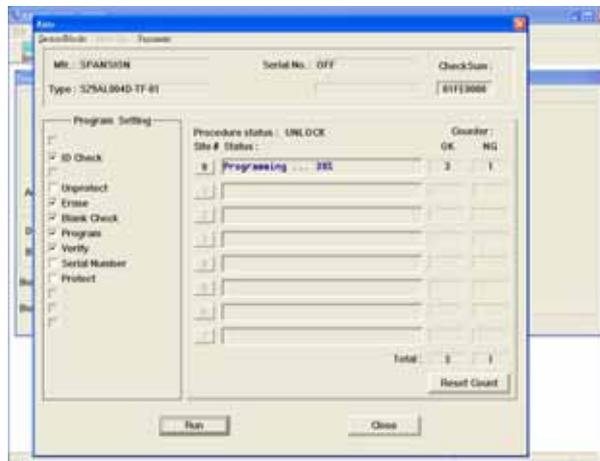
Click "Run" button on screen or "Y" key on keyboard or "YES" on programmer to start programming buffer contents to blank IC.
