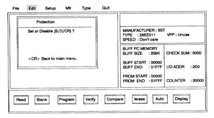
Press "S" to enable the protection or Press "D" to disable it, or press <CR> to return to the Edit menu.
