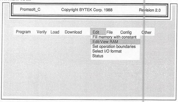
The Edit/View RAM command is a powerful screen oriented editor that permits viewing and changing of Programmer RAM contents. The editor operates on RAM blocks of 256 bytes each. You will be prompted for a starting address where editing should begin. If you simply press <enter> without entering an address, address 0000H will be selected as the default.
