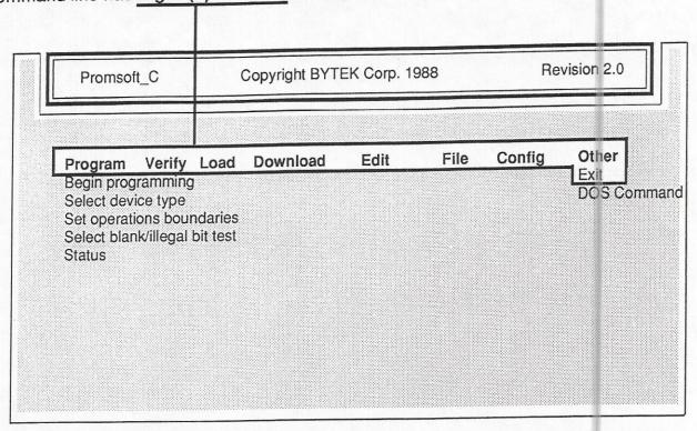
To Exit Promsoft\_C, simply press **ESC** key or select **OTHER** from the command line by either moving the cursor (highlighted area) or by pressing "O" followed by a return to accept the EXIT command and then respond "Y" (yes) to the prompt.
