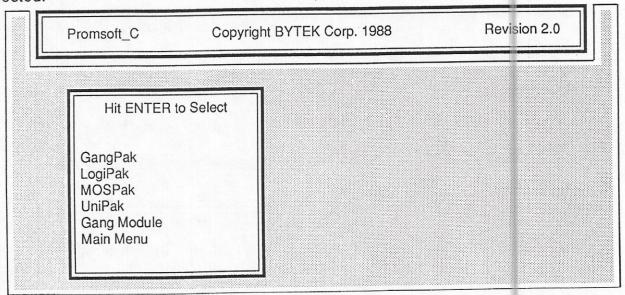
If you select an incorrect Cel/Program Pack type from this menu, Promsoft\_C may still seem to control the Programmer. Note, however, that messages displayed on the Promsoft\_C screen may be incorrect since messages are encoded by number and Programmers
