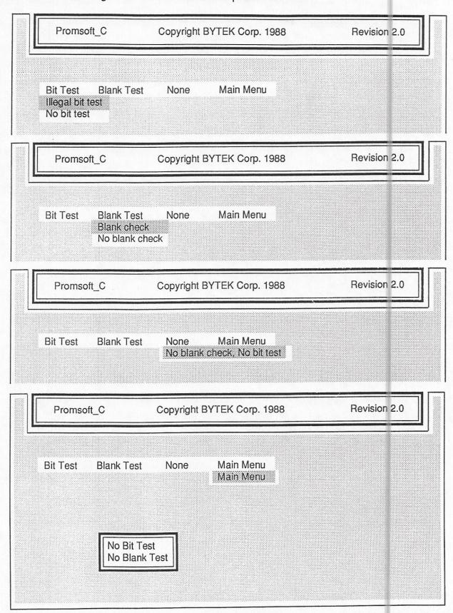
Briefly, an Illegal Bit Test tests the target device to ensure that the data in Programmer RAM should be programmable into the target device according to the programming rules and specifications of the currently selected device.
