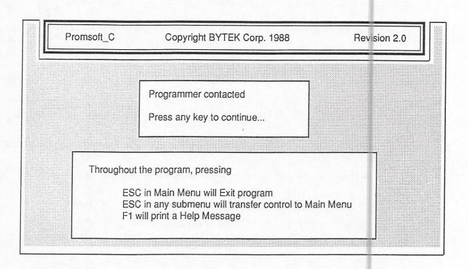
Assuming that the connection test passes, press any key to proceed to the Main Menu. If Promsoft\_C can not make connection with the programmer you will be prompted with a message: \_\_\_\_\_\_
