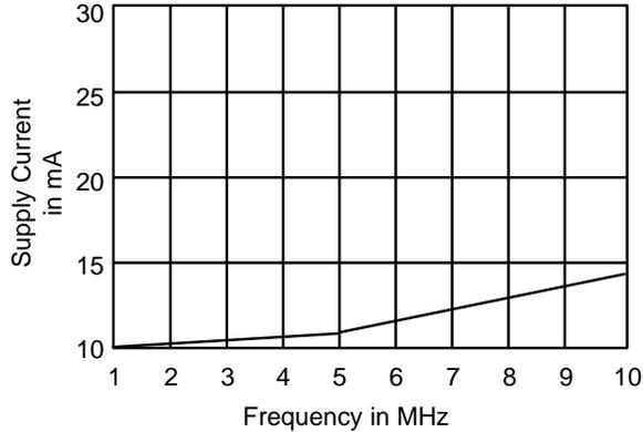
**Figure 1. Typical Supply Current vs. Frequency**
