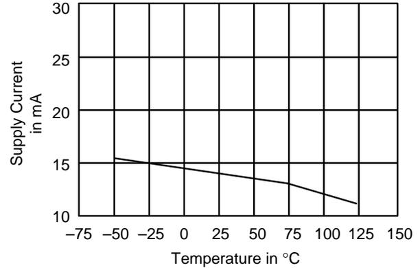
**Figure 2. Typical Supply Current vs. Temperature**
