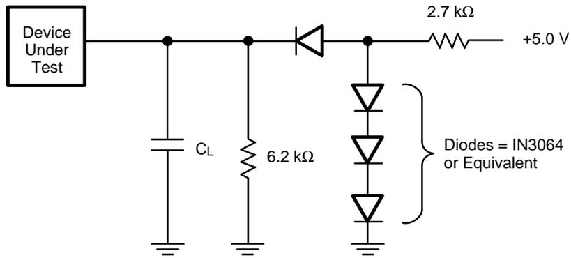
$C_L = 100 \text{ pF}$  including jig capacitance (30 pF for -55)
