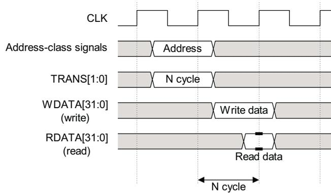
**Figure 3-2 Nonsequential memory cycle**
