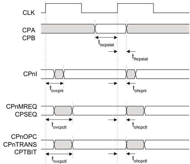
**Figure 8-2 Coprocessor timing**
