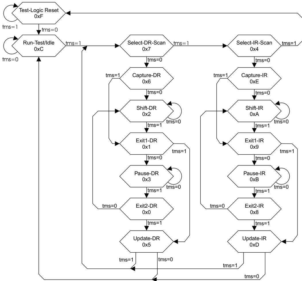
**Figure 5-8 Test access port controller state transitions**
