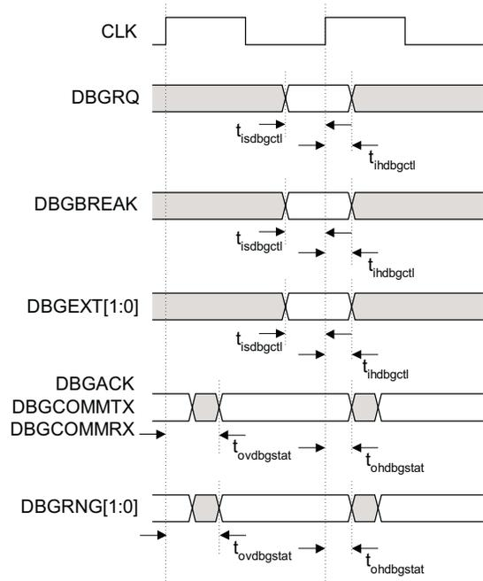
**Figure 8-4** Debug timing
