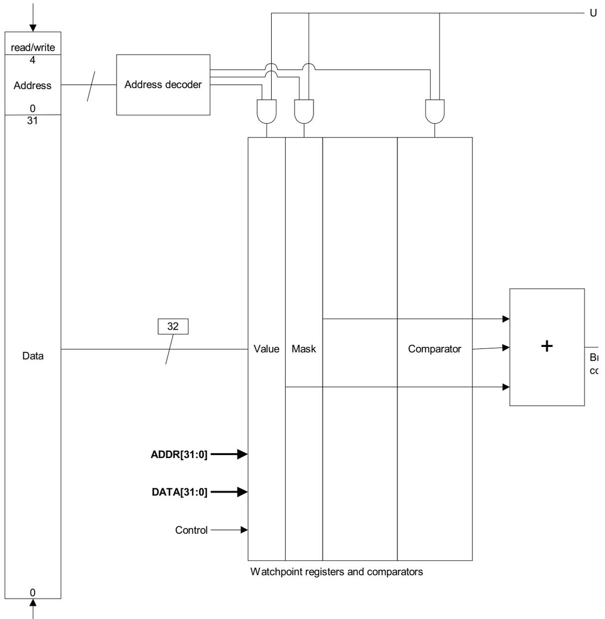
**Figure 5-12 EmbeddedICE-RT block diagram**
