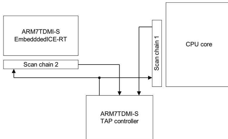
Figure 5-7 ARM7TDMI-S scan chain arrangements
