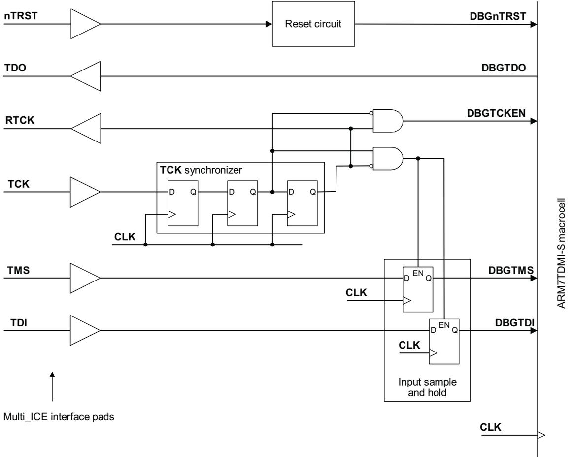
Figure 5-4 Clock synchronization
