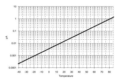
Figure 11 : Typical 'Zero Power' I<sub>DD</sub> vs. Temperature (V<sub>DD</sub> = 5.0V)
