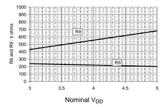
Figure 3c : Input Signal Amplifier, optimum values of R8 and R9 vs V<sub>DD</sub>
