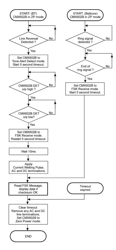
Figure 8c : Flow Chart for On-hook Operation of CMX602B
