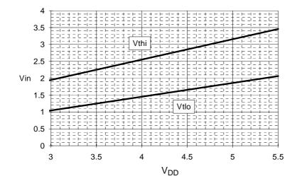
Figure 10 : Schmitt Trigger typical input voltage thresholds vs. V<sub>DD</sub>
