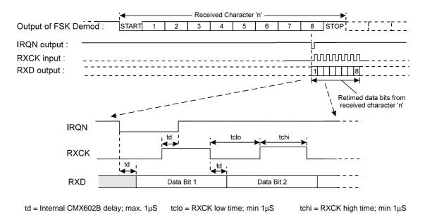
Figure 5a : FSK Operation With Data Retiming
