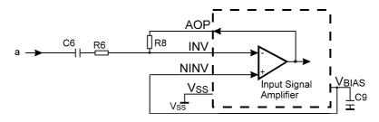
Figure 3b : Input Signal Amplifier, unbalanced input configuration
