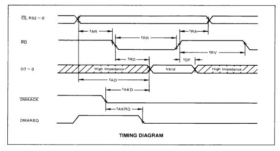
AC CHARACTERISTICS,  $(T_a = 0 \text{ to } 70^{\circ}\text{C}, V_{cc} = 5\text{V} \pm 10\%)$
