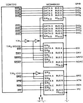
Note: In this example, high-speed data transfer cannot be made since the bus transceiver is of the open collector type (Set  $B_z\,=\,0$ ).
