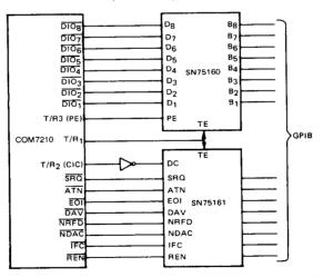
Note: In the case of low-speed data transfer ( $B_{\rm g}=0$ ), the T/R<sub>3</sub> pin can be used as a TRIG output. The PE input of SN75160 should be cleared to "0."
