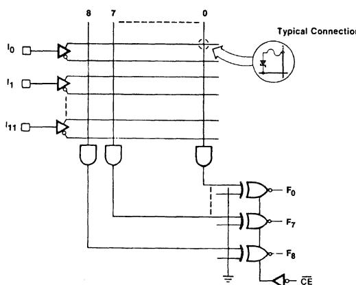
Fusible Ni-Cr links are initially intact at all array cross-points.
