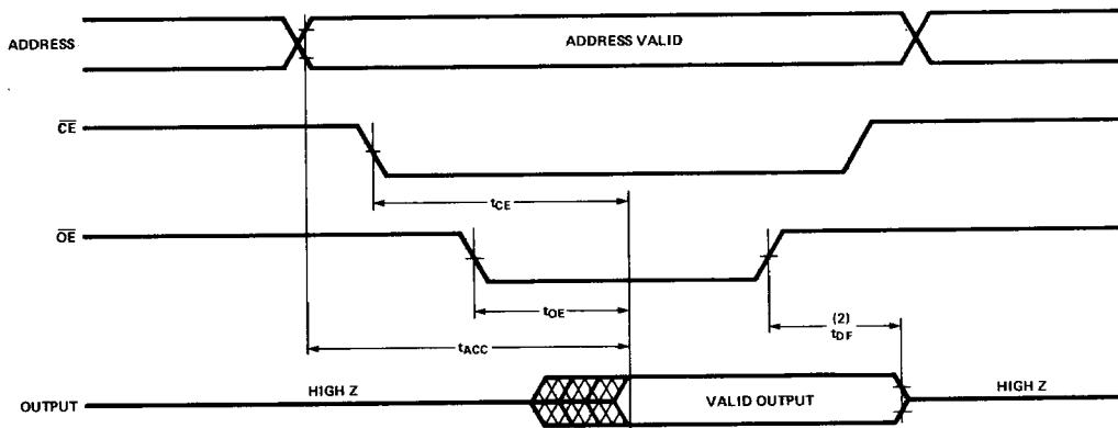
NOTE 2:  $t_{DF}$  IS SPECIFIED FROM  $\overline{OE}$  OR  $\overline{CE}$ , WHICHEVER OCCURS FIRST.
