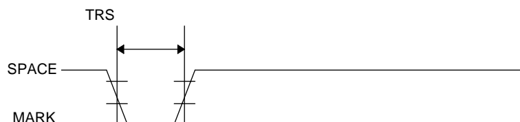
Figure 2.1.1 Minimum Reset Pulse Width (pin 6)
