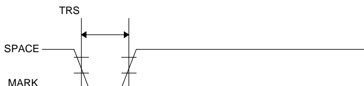
Figure 2.1.1 Minimum Reset Pulse Width (pin 6)
