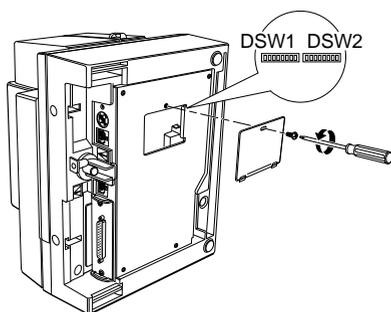
3. Set the switches using a pointed tool, such as tweezers or a small screwdriver.
