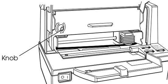
Make sure that the ribbon is installed below the print head without wrinkles or creases. (See ⑤ on the label for an illustration of where the ribbon should go.)
