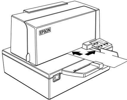
3. Insert the check straight into the paper inlet, using the right edge of the paper inlet as a guide.
