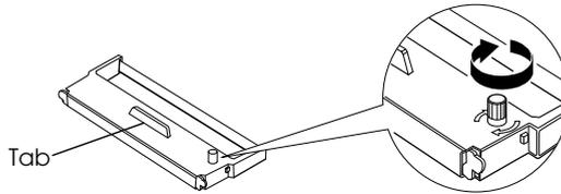
6. Insert the ribbon cassette in the printer and rotate the cassette's knob two or three more times. This is necessary to place the ribbon in the correct position.
