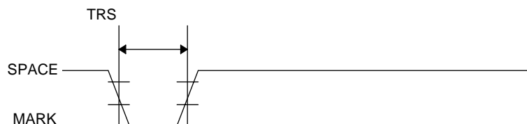
Figure 2.1.1 Minimum Reset Pulse Width (pin 6)
