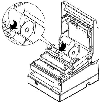
5. Tear off the paper on the cutter. If the paper was not fed far enough, press the RECEIPT FEED button to feed additional paper.
