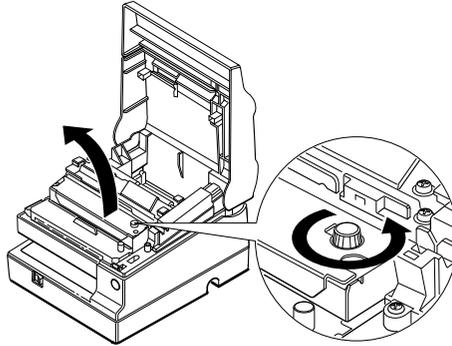
7. Remove any paper from inside the printer.
