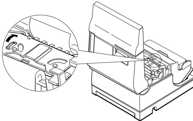
4. Move the OPEN <-> LOCK lever on each side of the printer in the direction shown in the illustration; the cutter unit then opens automatically.
