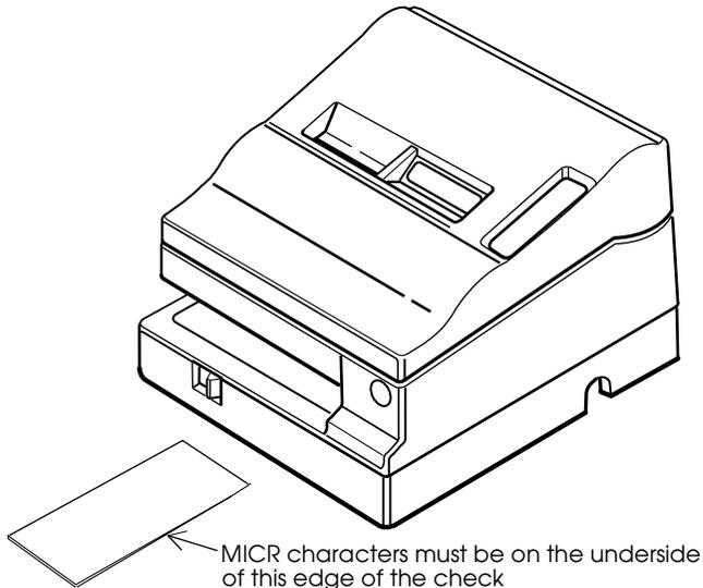
3. Insert the check straight into the paper inlet, using the right edge of the paper inlet as a guide.
