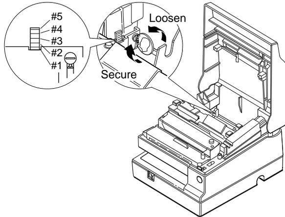
5. Loosen the adjusting screw with a coin or a screwdriver. Move the positioning plate to the appropriate position and then tighten the adjusting screw, as shown below. Position 1 leaves the least paper on the roll, and position 5 leaves the most
