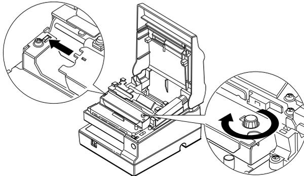
9. Close the cutter unit and lock it by moving both OPEN <-> LOCK levers in the direction shown in the illustration.
