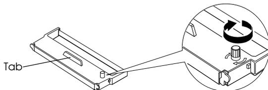
3. Insert the ribbon cassette in the printer and rotate the cassette's knob two or three more times as shown below. This is necessary to place the ribbon in the correct position.
