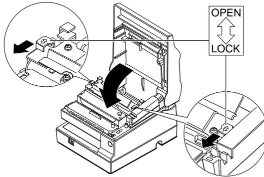
10. Install the paper roll following the steps in Chapter 1; then close the printer cover.
