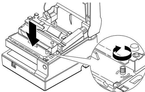
Make sure that the ribbon is installed in front of the print head without wrinkles or creases. If it is hard to see, open the print head cover as described in Chapter 3.
