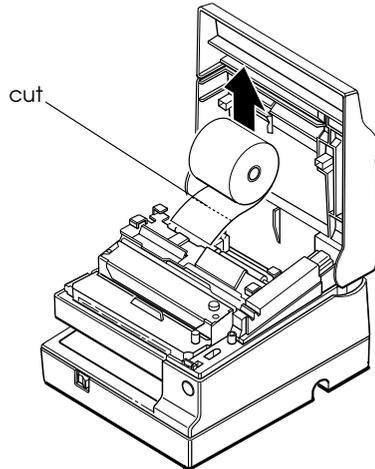
3. If the paper is caught in the automatic cutter blade, open the cutter blade by rotating the gear in the direction shown in the illustration.
