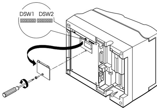
3. Set the switches using a pointed tool, such as tweezers or a small screwdriver.
