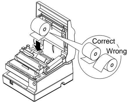
4. Insert the tip of the paper into the paper inlet and push it in until it is automatically detected and fed into the printer.
