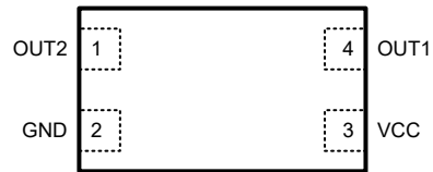
Figure 5-2. ZFC Package, 4-Pin X1LGA (Top View)
