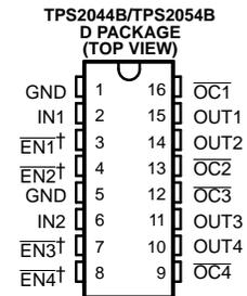
† All enable inputs are active high for the TPS205xB series.
