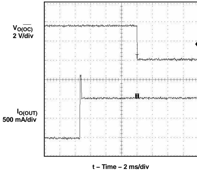
Figure 8. 3- $\Omega$  Load Connected to Enabled Device
