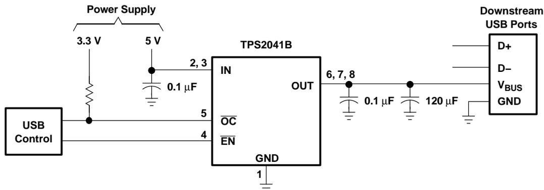
Figure 30. Typical One-Port USB Host / Self-Powered Hub
