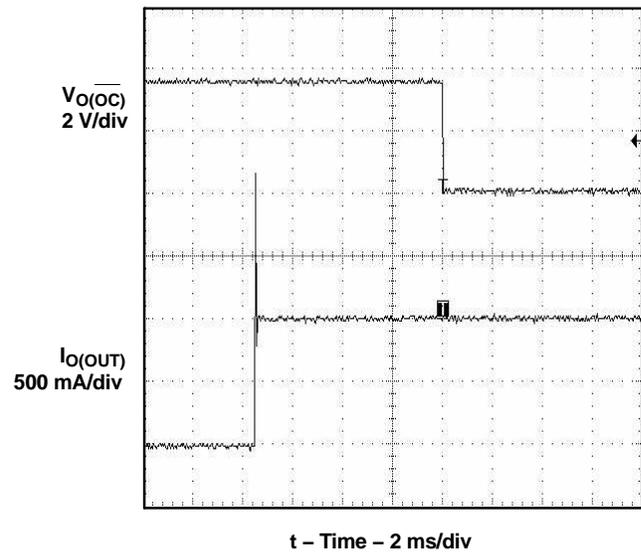
Figure 9. 2- $\Omega$  Load Connected to Enabled Device
