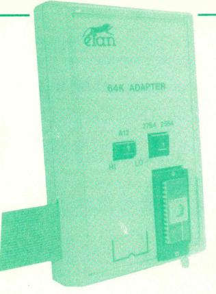
The E6 provides a simple and economic extension to facilities of earlier models of 24 pin socket programmers to accommodate 64K bit EPROM devices.
