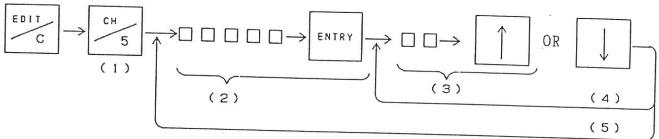
(1) Press the "CH" switch to activate the CHange mode. Pressing the "CH" switch will display address "0" and the contents of the RAM.
