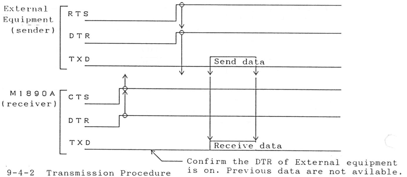
The 1890A supports the two data communication control procedures:
