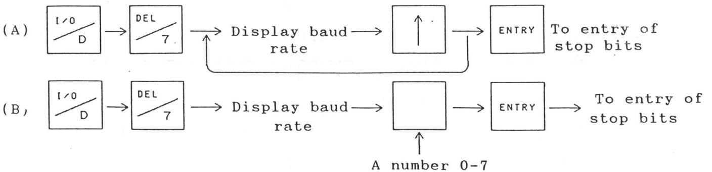
(A) is the way to select the baud rate by "↑" key and (B) is the way to select the baud rate directly by entering the number.
