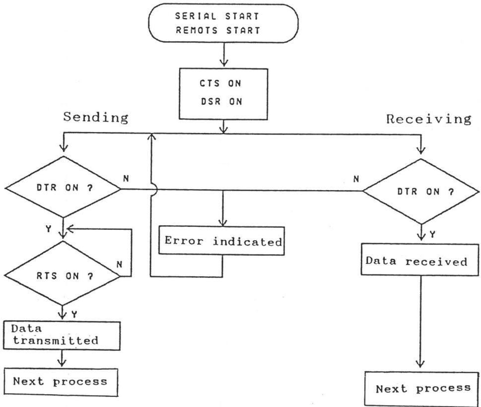
A communication interface IC equivalent to the 8251A is employed in the RS232C interface of the Model 1890A.
