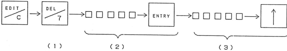
(1) Press "DEL" switch to access the DELETE mode.
