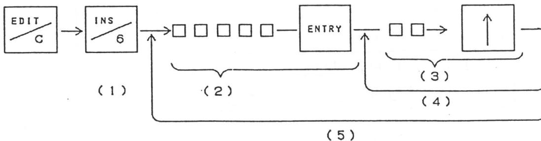
(1) Press "INS" switch to activate the INSert mode.
