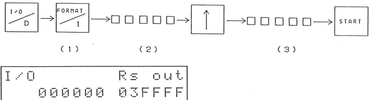
(1) Specify the output port of data: RS232C by "1" and Parallel by "3".
