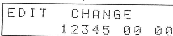
(3) Enter new data of two digits. Pressing "↑" switch will cause the data entry to be written on the buffer memory and the next address and the data to be appear on the display.
