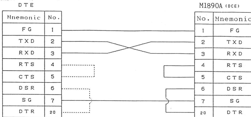
NOTE: The connector pin assignments as DTE are specified by the RS232C standard. Therefore, if DCE equipment are connected to each other using a 1:1 cable, satisfactory results cannot be obtained.
