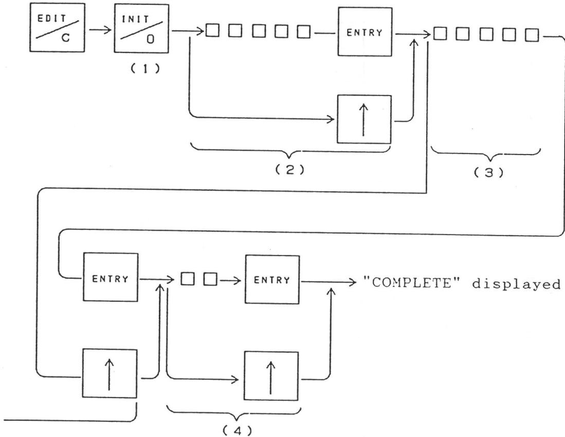
(1) Press "INIT" switch to active the INITIALize mode. The programmer will display the following message with the starting address 0.
