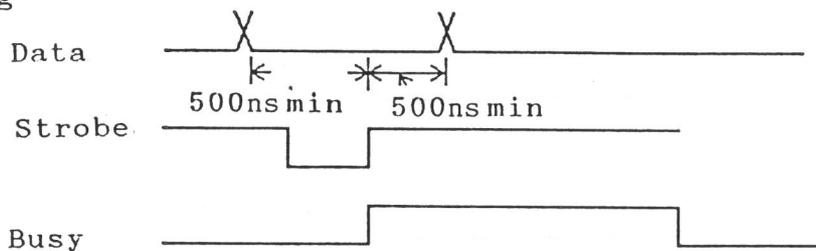
In the 1890A system, data is input at the leading edge of the strobe signal. Once data has been input, the busy signal will output for a certain period of time. Thus, the sender must output data and the strobe signal when the busy signal is in the state of "0".
