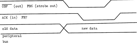
The output buffer full signal,  $\overline{\text{OBF}}$ , is an active low strobe generated by the EP8000 and should be used to strobe data into the peripherals input latch.  $\overline{\text{OBF}}$  returns high when the answering acknowledge signal, ACK is also high. The ACK signal is an active high signal issued by the peripheral used to tell the EP8000 that data has been latched into the peripheral's buffer. ACK returns low when the peripheral requires the next transaction to take place.
