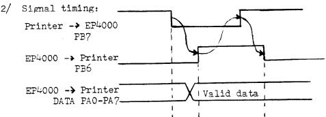
PB7 is set low by the printer when it is ready to receive data.
