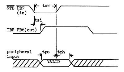
tsw STB pulse width 300ns typical tsi STB to IBF delay 200ns typical tps data setup 150ns typical tph data hold 50ns typical
