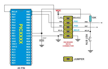
After programming device development are finished, the male IDC10 connector pins must switched by jumpers. enables pins MCLR, RB6 and RB7 to be connected to the rest of on board electronics, which further enables device to operate normally without PICflash programmer. In case of need, the jumpers can be removed and PICflash can be reconnected for reprogramming the chip.
