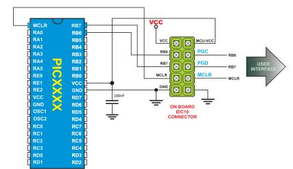
Connection schematics for male IDC 10 connector on printed board and 40-pin 16F and 18F PIC microcontrollers. Some of the examples are:
