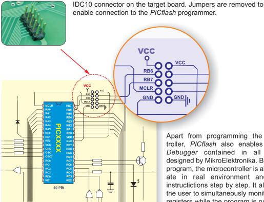
enable connection to the PICflash programmer.
