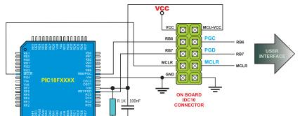
Connection schematics for male IDC 10 connector on printed board and 64-pin 18F PIC microcontrollers. Some of the examples of 18F family:
