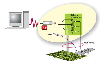
By clicking the WRITE option, multiplexer within the programmer disconnects the microcontroller pins from the rest of electronics on the board. It allows programming of the microcontroller by using PGC, PGD and MCLR signals. When programming completed, *PICflash* automatically changes its state and becomes inactive.
