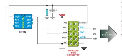
Connection schematics for male IDC 10 connector on printed board and 8-pin 12F PIC microcontrollers. Some of the examples of 12F family:
