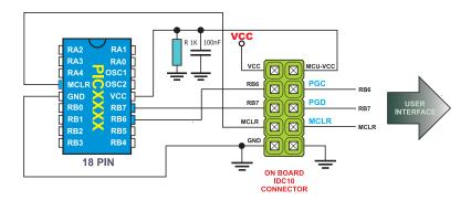
Connection schematics for IDC 10 mail connector on printed board and 18-pin 16F PIC microcontrollers. Some of the examples of 16F family:
