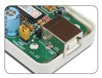
This picture illustrates the position of jumper when the target board and programmer are powered via USB cable.
