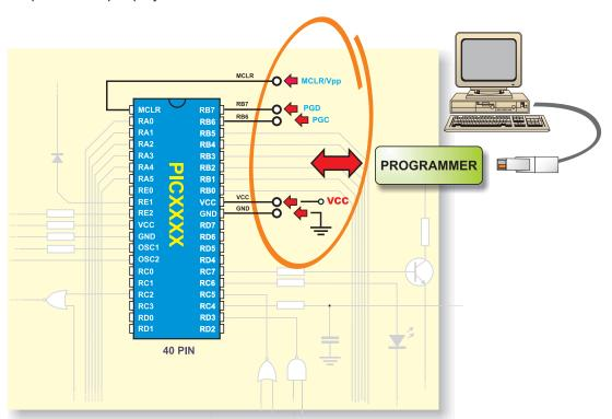
Since the microcontroller is soldered on the printed board (with no use of socket), it is necessary to switch these pins by using jumpers. In consequence of that, on device designing, do not forget to provide space for embedding 5 jumpers. They should be embedded between pins for programming and components connected to these pins.
