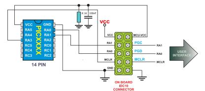
Connection schematics for male IDC 10 connector on printed board and 14-pin 16F PIC microcontrollers. Some of the examples of 16F family:
