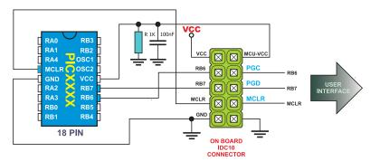
Connection schematics for IDC 10 mail connector on printed board and 18-pin 18F PIC microcontrollers. Some of the examples of 18F family:
