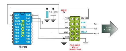
Connection schematics for IDC 10 mail connector on printed board and 20-pin 16F PIC microcontrollers. Some of the examples of 16F family:
