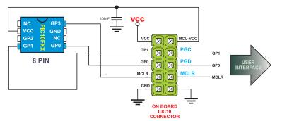
Connection schematics for male IDC 10 connector on printed board and 8-pin 10F PIC microcontrollers. Some of the examples of 10F family:
