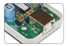
This picture illustrates the programmer with no jumper for power supply selection. In this case the programmer is powered by the target board which has its own power supply.
