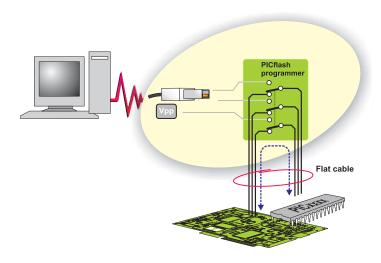
A multiplexer within the programmer connects the microcontroller pins to peripheral components on the printed board via *flat* cable. In that way, the microcontroller directly controls the operation of device with no impact of the programmer. Accordingly, even the IDC10 connector is connected, the *PICflash* programmer does not affect device operation.
