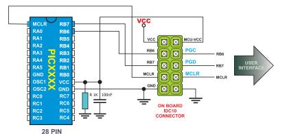
Connection schematics for male IDC 10 connector on printed board and 28-pin 16F and 18F PIC microcontrollers. Some of the examples are:
