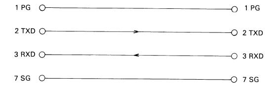
NOTE: Some machines do not have internal pull-ups and require extra connections within the cable form. Pull-ups may be required on pins 5, 6 and 8 of the external device if it is DTE or pins 4, 6 and 20 if it is DCE.
