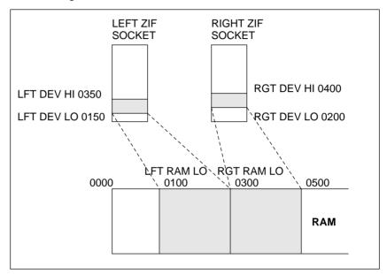
There are two address limits which can be selected for a single device, these are called Address Low (0150) and Address High (0350). When two devices are in use this figure becomes four as an Address Low (0200) and an Address High (0400) can be specified on the second device.
