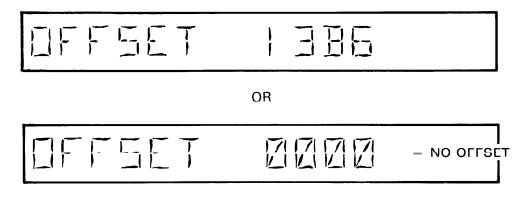
By use of the keyboard the new offset can be entered: e.g. offset 1A00.
