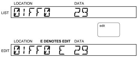
The data '29' at location '01FF0' can now be changed by use of the hex keyboard into for instance A3:
