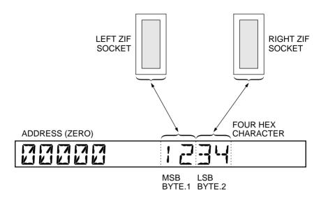
(Under the 'List' function THE ADDRESS RANGE can be scanned by use of the hex keyboard and cursor keys) see section 'LIST'.
