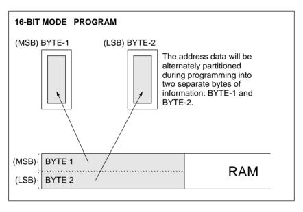
MSB – The most significant BYTE in binary code LSB – The least significant BYTE in binary code
