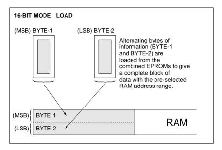
MSB – The most significant BYTE in binary code LSB – The least significant BYTE in binary code
