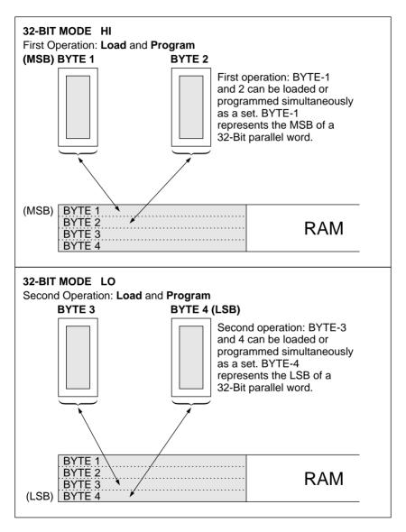
MSB – The most significant BYTE in binary code. LSB – The least significant BYTE in binary code.
