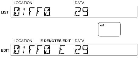
The data '29' at location '01FF0' can now be changed by use of the hex keyboard into for instance A3:
