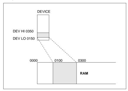
There are two address limits which can be selected for a single device, these are called Address Low (0150) and Address High (0350).
