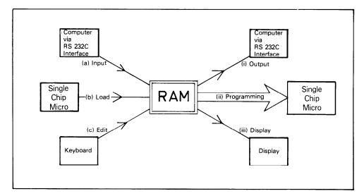
Data can be loaded into the Ram of the PP39 from 3 different sources, these are:
