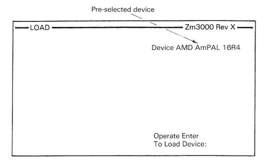
Press the ENTER key and the display will first show ''loading'' in progress and then ''Device Loaded'' indicating that the operation is complete.
