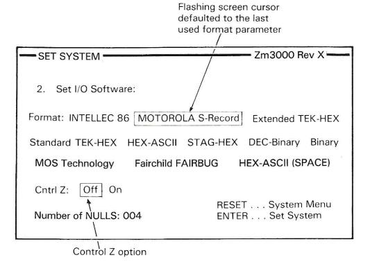
Nine format parameters are available. Selection can be made by use of the horizontal cursor keys which direct the screen cursor from the last entered selection to the required alternative.
