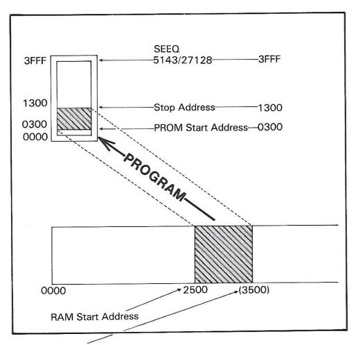
No stop address is entered for the RAM as data programmed will automatically default to the size of the data block specified within the device.
