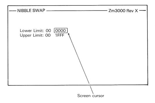
Interchange between the limits is made by using the cursor keys and new values can be entered from the hex-keyboard. To confirm the address limits:
