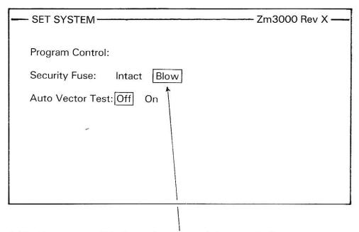
A Flashing cursor will indicate the status of the security fuse feature.
