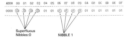
Before the second device can be programmed, the RAM data within the specified limits of 0000 to 00FF must first undergo NIBBLE SWAP:
