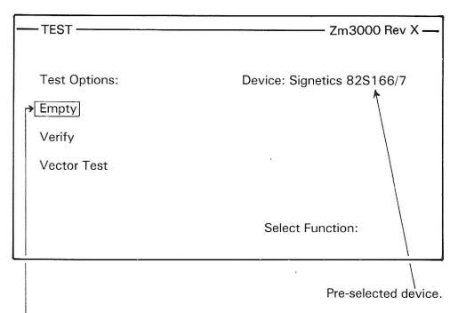
The screen cursor will indicate the "EMPTY TEST" default condition. The "VECTOR TEST" can be selected by pressing the down cursor key twice.
