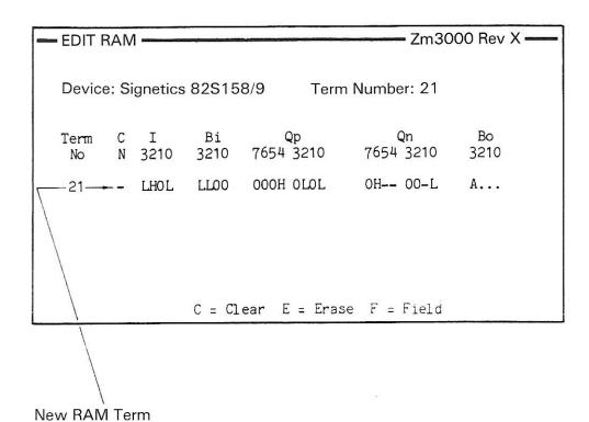
More Terms can be displayed for Editing by pressing either of the vertical cursor keys, by directly entering a two digit Term number or by pressing one of the command keys 7, 8, 9, E or A.
