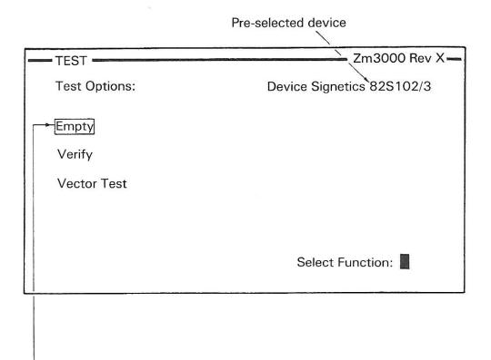
The screen cursor will indicate the "EMPTY TEST" default condition. The VERIFY TEST can be selected by the down cursor key.
