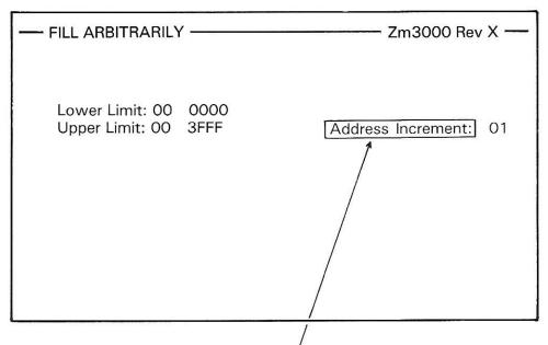
The screen cursor shows the Address Increment in the default state of 1. If an Address Increment other than 1 is required it can now be entered directly from the keyboard and can take values from 1 to 8.
