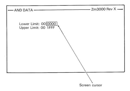
Interchange between the limits is made by using the vertical cursor keys and new values can be entered from the hex-keyboard.
