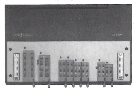
The Zm3000 Universal Programming Station is equipped with 8 ZIF sockets which enable it to program the vast majority of programmable devices in every technology. An optional SMD Chip Station is available to allow programming of PLCC and LCC equivalents of DIP devices supported by the Zm3000. The SMD Chip Station plugs into the DIN connectors at either end of the Zm3000.
