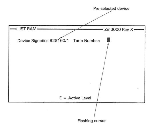
The display shows a flashing cursor indicating that a Term Number should be entered to display a section of array.
