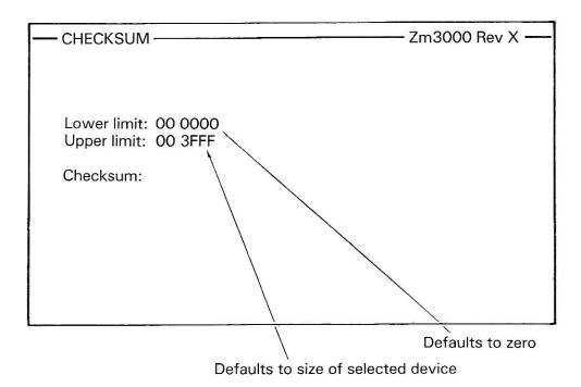
Address limits can be independently selected for the manual checksum (unlike the automatic versions which default to limits pre-selected in their respective operations i.e. Program, Load, Verify etc). Interchange between the two limits is made with the vertical cursor keys and new selections can be entered from the hex-keyboard.
