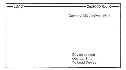
**Note:** Should a PAL's security fuse be blown it will not be possible to load its fuse pattern into the programmer.
