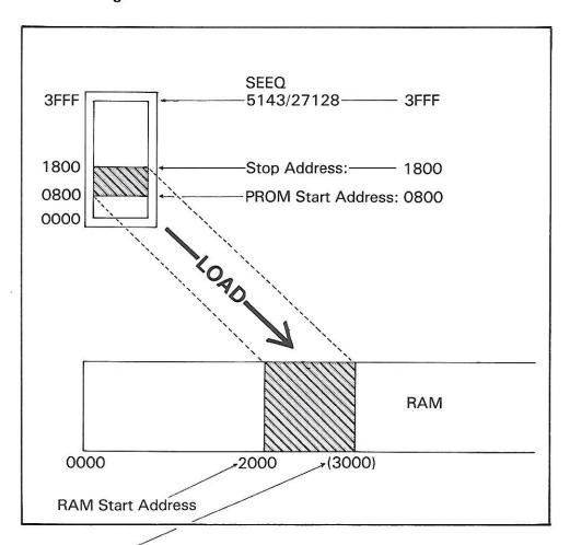
No stop address is entered for the RAM. Data loaded will automatically default to the size of the data block specified within the device.
