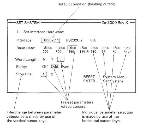
Entry into a particular parameter category is made by use of the vertical cursor keys and is indicated by the applicable screen cursor flashing.
