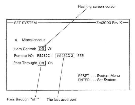
If, as in this example the RS232C 2 port was previously used in REMOTE MODE and RS232C 1 is the new requirement, then it can be selected as follows:
