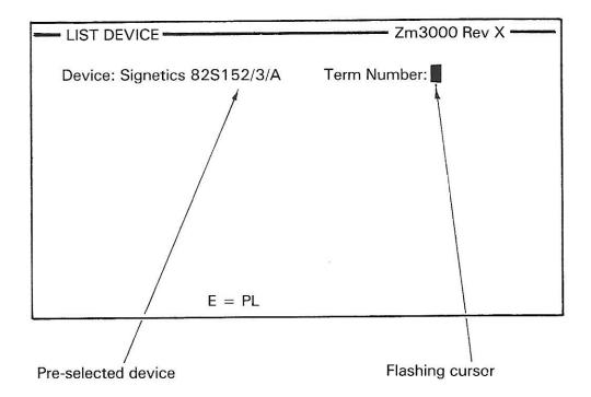
The display shows a flashing cursor indicating that a Term Number should be entered to display a section of fuse array.
