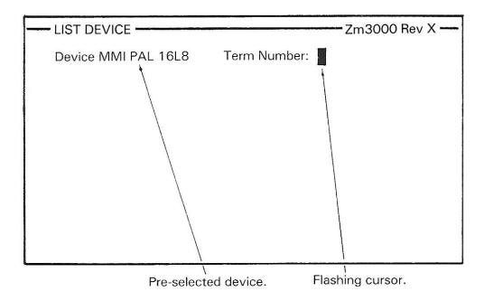
The display shows a flashing cursor indicating that a term number should be entered to display a section of fuse array.
