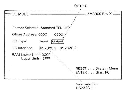
In some circumstances, the static screen cursor indicating the last used serial port will move onto the alternative serial option simultaneously with selection of either INPUT or OUTPUT.
