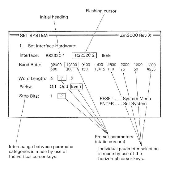
Entry into a particular parameter category is made by use of the vertical cursor keys and is indicated by the applicable screen cursor flashing.
