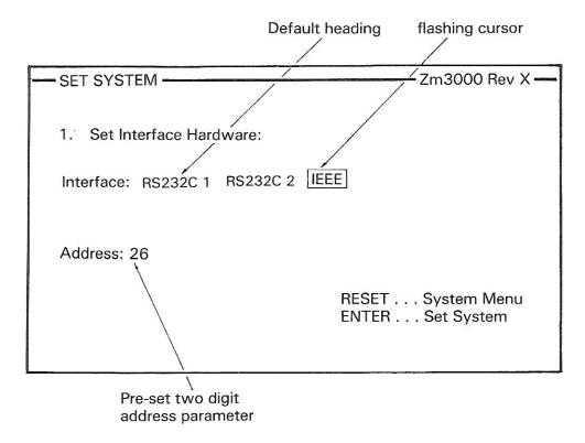
Pressing the down cursor key will make the address available for selection, indicated by the pre-set parameter flashing. The new address can now be entered from the keyboard. To confirm this selection:
