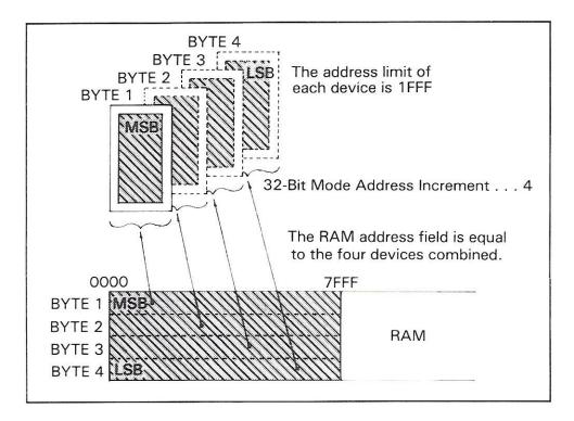
In the first operation: PROGRAM or LOAD is made to and from a single 8-Bit device with only BYTE 1 the ''most significant byte'' of a 32-Bit Word undergoing data transfer.
