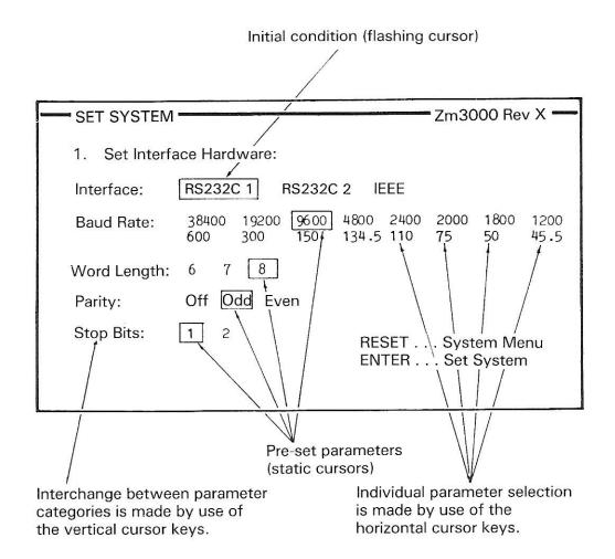
The flashing screen cursor will be initially on the heading RS232C 1, and four static cursors will indicate the previously entered I/O parameters for this particular port.
