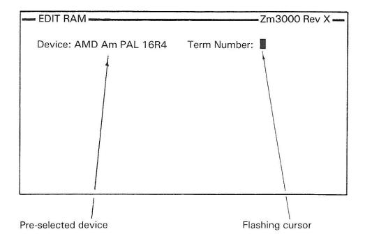
The display shows a flashing cursor indicating that a two digit number should be entered to display a single Term.
