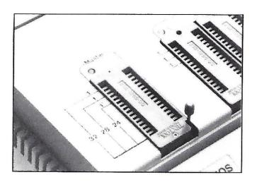
Device inserted.Socket open.
