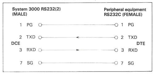
Note: Some machines do not have internal pull-ups and require extra connections within the cable form. Pull-ups may be required on pins 5, 6 and 8 of the external device if it is DTE or pins 4, 6 and 20 if it is DCE.
