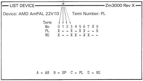
The programmable Polarity and Register operate interactively within the Output Macro Cell to produce one of four modes, as listed below:
