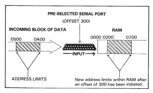
A more widely used example occurs when an offset is specified so that the start address of the incoming block of data becomes zero in the RAM.
