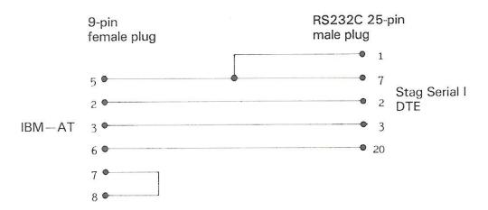
IBM-AT connected to the male (serial II) interface on a Stag programmer
