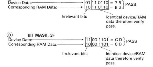
7F tends to be the most commonly required BIT MASK as it is associated with the ASCII code.
