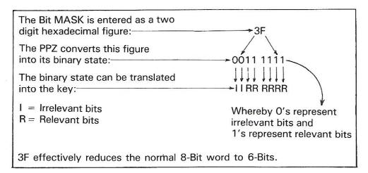
This means that the two most significant bits of the 8-Bit word can be either 0 or 1.
