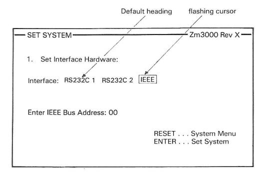
Pressing the down cursor key will make the address available for selection, indicated by the pre-set parameter flashing. The new address can now be entered from the keyboard. To confirm this selection:
