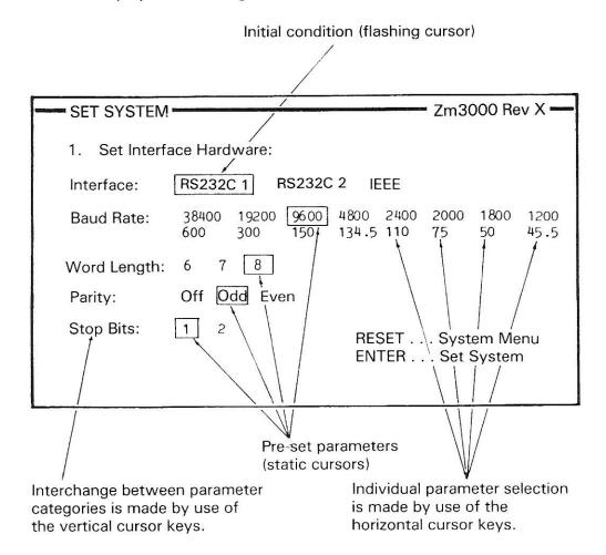
The flashing screen cursor will be in its default state on the RS232C 1 heading. To select the RS232C 2 category.
