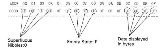
As can be seen from the above section, the data displayed in each individual location is in the form of bytes. However, the left nibbles containing 'O's' are superfluous throughout the entire device address range. Only the right nibble reflects the condition of the 4-Bit device. In this case the empty state—'F'.
