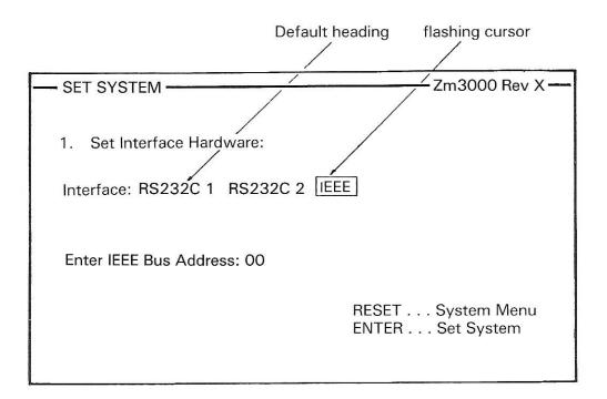
Pressing the down cursor key ( $\downarrow$ ) will make the address available for selection, indicated by the pre-set parameter flashing. The new address can now be entered from the keyboard. To confirm this selection:
