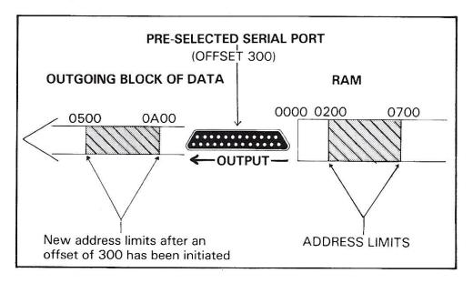
A more widely used example is when re-location to a higher address occurs from a start address of 0000 in the RAM.
