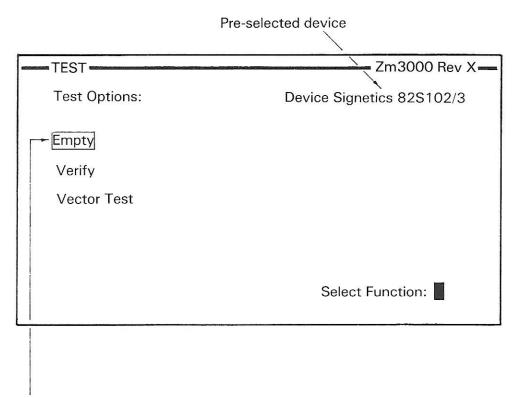
The EMPTY TEST is the default condition of TEST and is indicated by a screen cursor.
