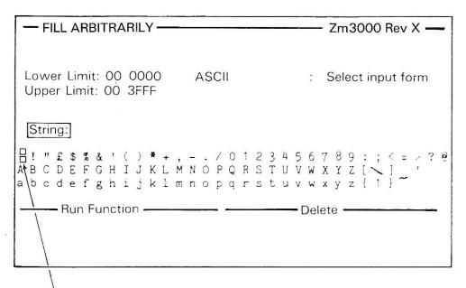
The screen cursor will now be in the default position on the space character. By using all of the cursor keys, any character from within the ASCII register can be pin pointed and then selected by pressing the ENTER key.
