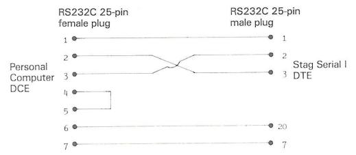
IBM-PC connected to the male (serial II) interface on a Stag Programmer.
