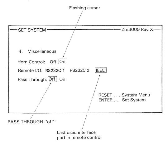
Selection of PASS-THROUGH can now be made by pressing the down cursor key twice which will transfer the flashing screen cursor onto "pass through: off".
