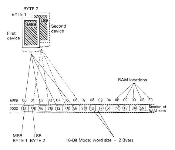
MSB—The "most significant BYTE" in binary code LSB—The "least significant BYTE" in binary code
