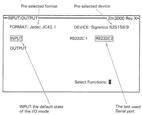
INPUT is the default state of the I/O mode, OUTPUT can be selected by use of the down cursor key.
