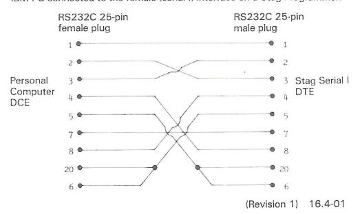
IBM-PC connected to the male (serial II) interface on a Stag programmer.
