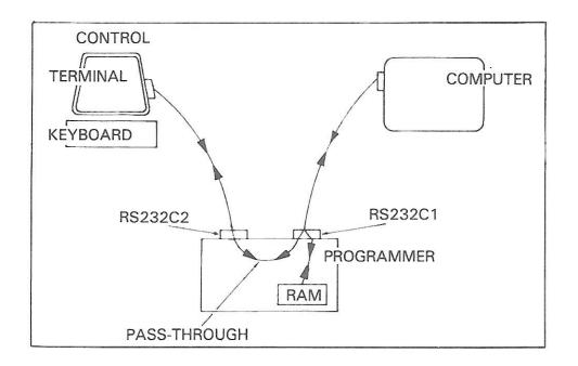
In effect PASS-THROUGH duplicates the operating structures as shown below.
