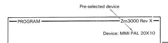
Pressing the ENTER key will implement the program sequence. This includes a series of automatic checks on the RAM and the device.
