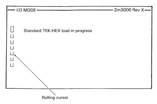
**NB:** Transmitted data that falls outside the boundaries of any pre-selected RAM limits will still be indicated during the INPUT operation by the rolling cursor but will not affect the RAM.
