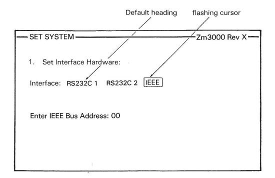
Pressing the down cursor key ( $\downarrow$ ) will make the address available for selection, indicated by the pre-set parameter flashing. The new address can now be entered from the keyboard. To confirm this selection:
