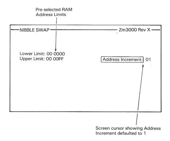
If required by the user, the nibble swap function on 4-bit devices can be integrated with Address Increment to handle data in the 16-bit mode and beyond.
