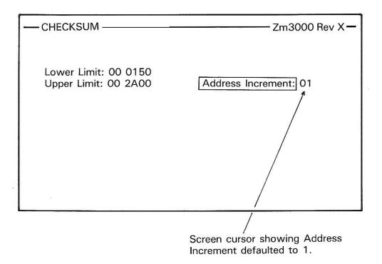
If an Address Increment other than 1 is required it can now be entered from the keyboard. (See Section 3 for further details.)
