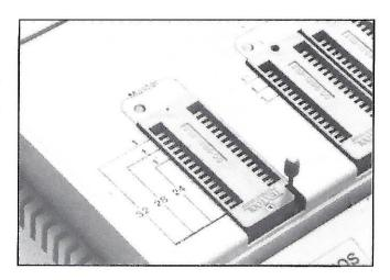
Device inserted.Socket open.
