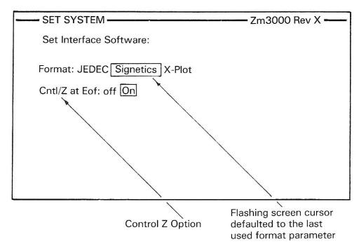
The display shows a flashing screen cursor defaulted to the last used Format Parameter plus a second static cursor indicating the availability of the Control Z option.
