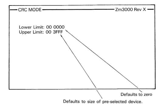
Both Upper and Lower Address Limits can be changed, and also an Address Increment can be selected as with CHECKSUM.
