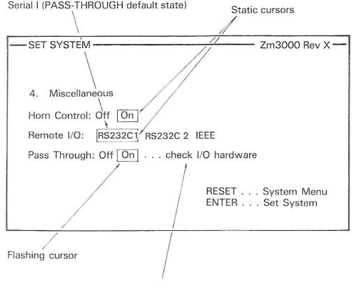
The display will also show a visual reminder to check that the System 3000's 'I/O hardware' i.e. Baud rate, Parity, etc., correlate for both serial interface ports during PASS-THROUGH.
