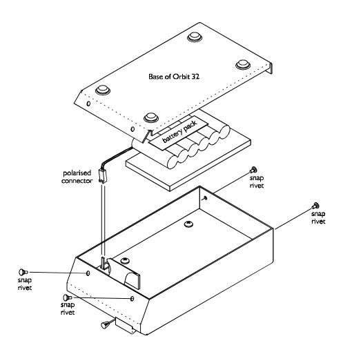
Dissassembly of Orbit 32 to remove battery pack
