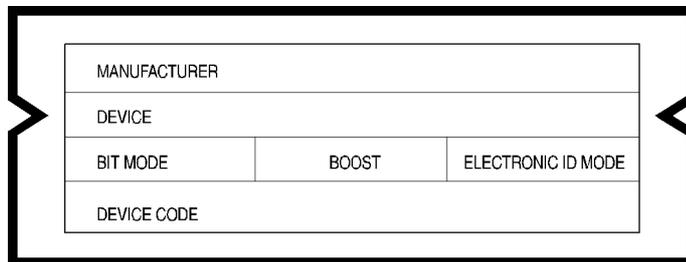
The BOOST message is only displayed when the Orbit 48 is on boost charge, during which time, no device functions may be executed.
